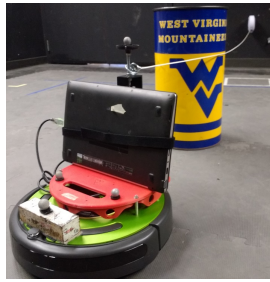
Fig. 4. Tethered robot used in the experiments of this paper.
